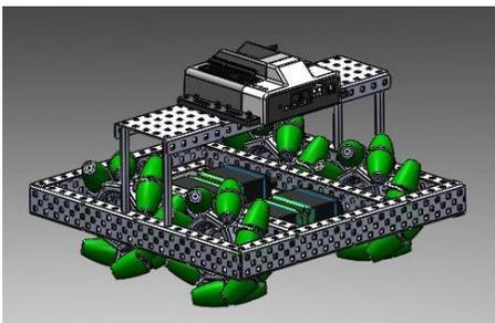
Figure 2: Robotic Chassis with Motor Mecanum Drive
